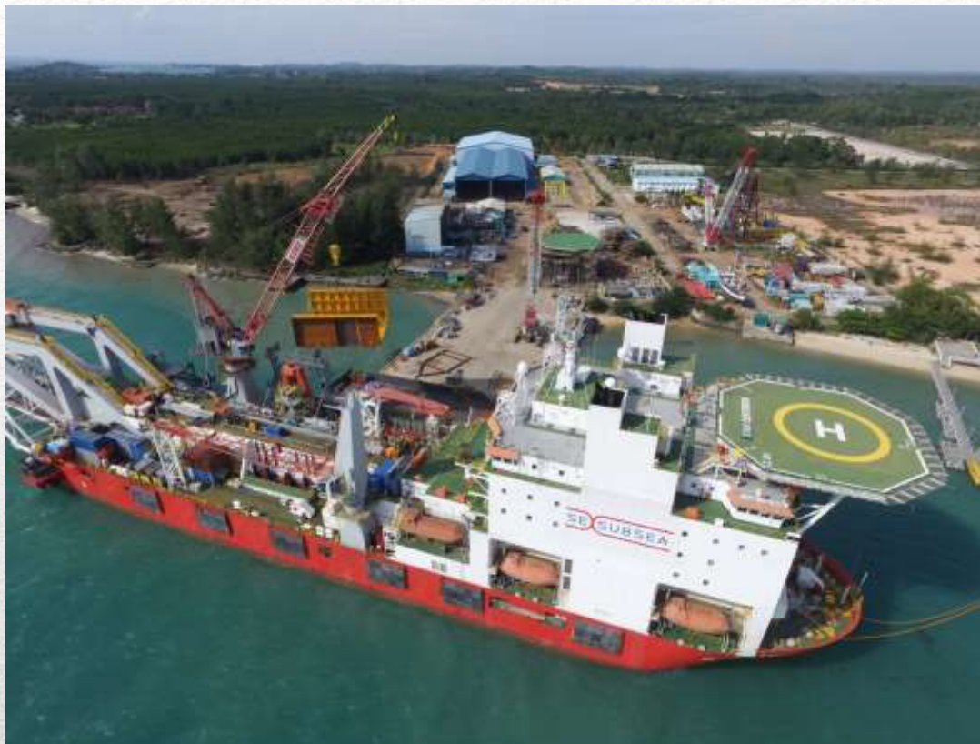
Pipelay Vessel “Star Centurion” [GT: 27082, LOA 144m]
